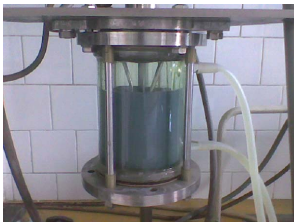
Figure 1. Homogeneity of the polymer-MWCNT nanocomposite latex achieved after using miniemulsion polymerization (latex based on SAN synthesized in the presence of 2% CNTs). [Color figure can be viewed in the online issue, which is available at wileyonlinelibrary.com .]
